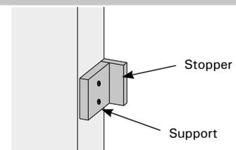
**5.** Fix one side of the frame to the opening with screws (topmost screw first). Place wedges next to bores between the supports. Make sure the wedges are not placed under the bores.
