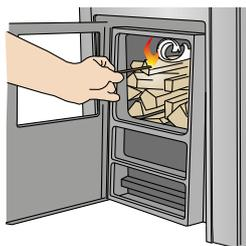
If you start the fire under the firewood, all the wood will heat up and gasify simultaneously. If this happens, the air in the chamber is not sufficient for controlled burning and some of the gas flows into the chimney and escapes outside without burning. This requires more wood and causes more emissions. Too slow combustion is also a bad alternative, because it does not allow the temperature to rise high enough and the burning is not efficient.
